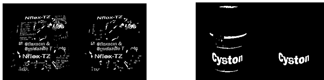
Figure 3.13 Image represents the difference in a medicine strip image and a bottled medicine, before and after region filtering ( I_3 ). The geometric checks have considerably reduced the number of non-text regions, when compared with the previous image.
