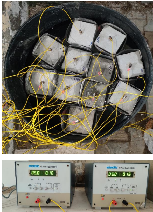
Figure 4.4: RC specimens subjected to accelerated impressed current for corrosion studies
