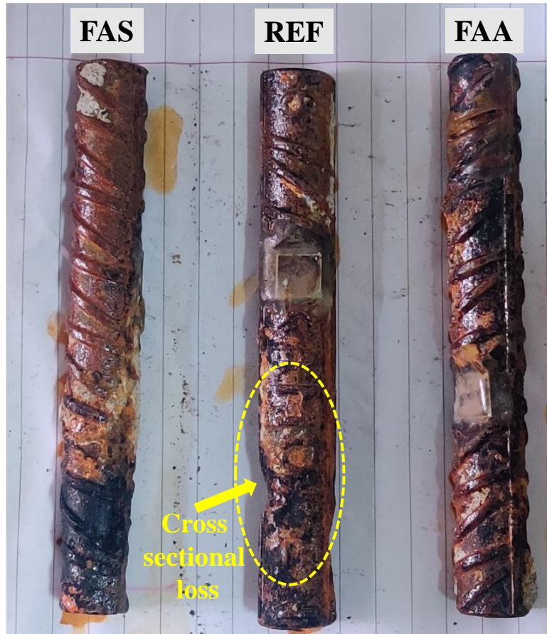
Figure 4.15: Condition of rebar extracted from the tested specimens
