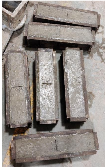
Figure 5.1: Artificial cracks generated in prismatic specimens during casting
