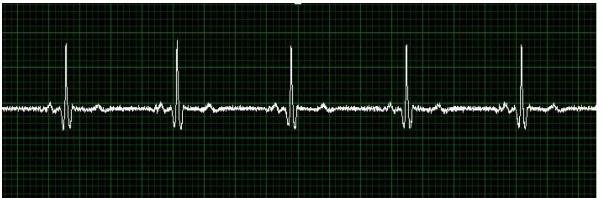
Figure 4.5 ECG signal after remove Baseline Wandering
