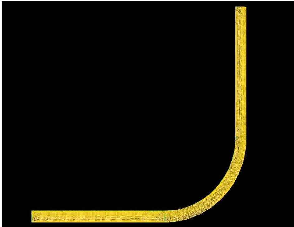
Figure 5.2: Meshed Pipeline Bend
