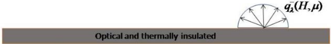
Fig- 3.7 schematic of insulated wall bottom surface of the receiver
