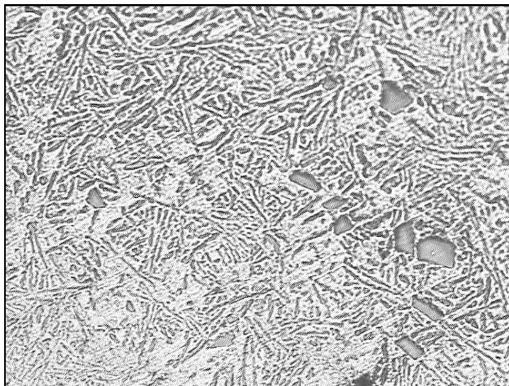
Figure 6.6: Micrograph of Sample-1 Al-12.6%Si at 200X.
