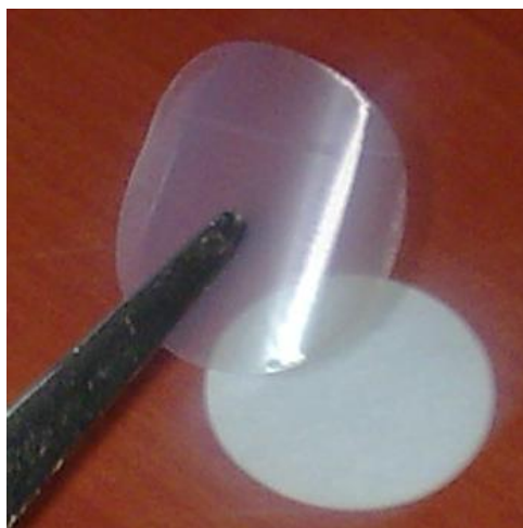
Figure 5.1: Image of the polycarbonate membrane used for electrochemical template synthesis
