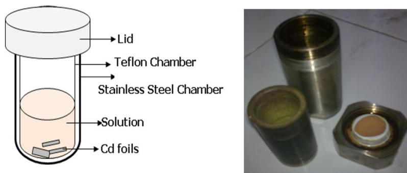
Figure 6.1: Schematic and the pictorial view of the teflon-lined stainless steel chamber used in solvothermal synthesis
