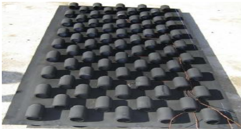
Fig 2.5 Absorber plate used in collector with obstacles (Ozgen et al 2009)
