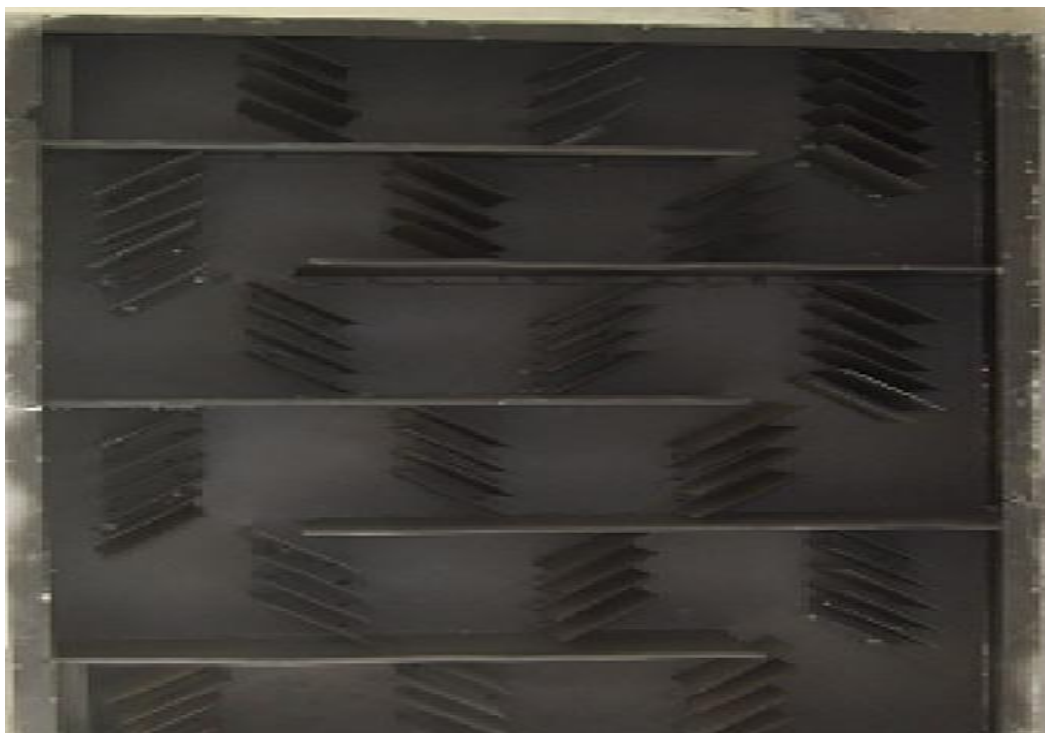
Fig.2.4.Rectangular obstacles inclined at 45 0 (Akpinar and Kocyigit 2010)
