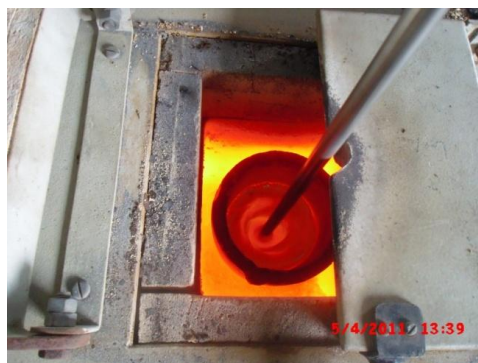
Figure 1.13: Stir casting set up
