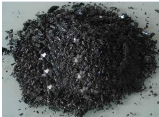
Figure 1.16: Silicon Carbides as reinforcement [10]
