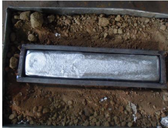
Figure 4.10: Mould and cast product after casting
