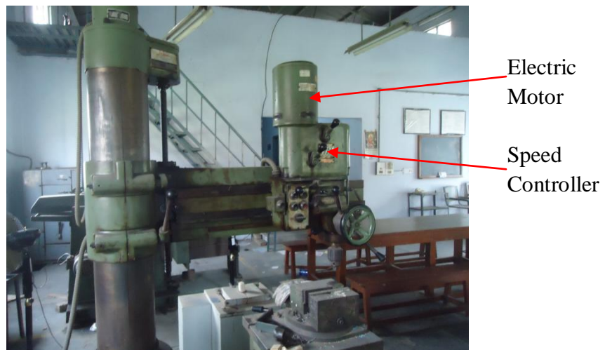
Figure 4.7: Drilling Machine used for Stirring Purpose
