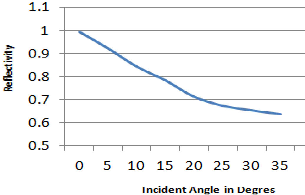
Fig 4.3 Simulated for TE- HCG with grating period ( \Lambda ) = 1170 nm, thickness ( t_g ) = 340 nm, duty cycle ( \eta ) = 0.65. Wavelength = 1550 nm.
