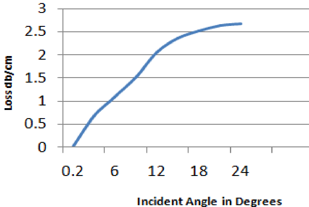
Fig.4.5 Simulated for TE- HCG with grating period ( \Lambda ) = 1170 nm, thickness ( t_g ) = 340 nm, duty cycle ( \eta ) = 0.65. Wavelength = 1550 nm
