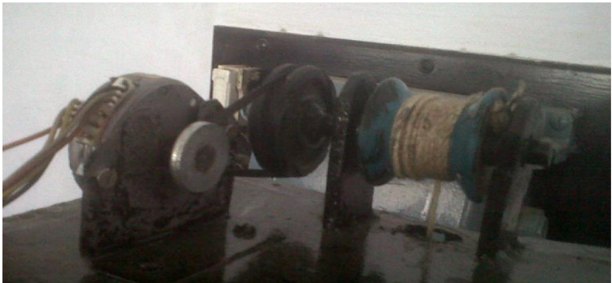
FIGURE 3.12 STEPPER MOTOR CONNECTED WITH ELEVATOR LIFTING PULLEY
