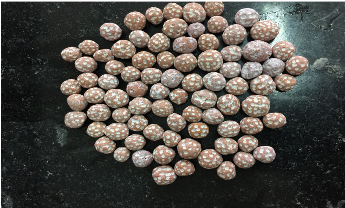
Figure 5.3(b): Used TiO 2 coated clay beads.
