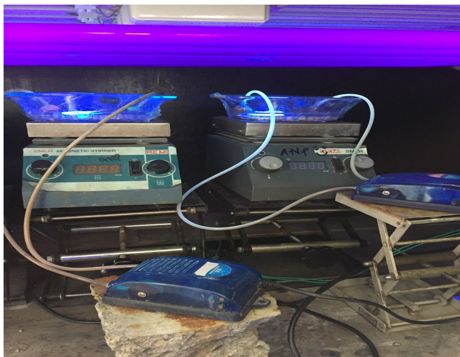
Figure 5.4: Lab-scale setup of fixed-bed reactor.
