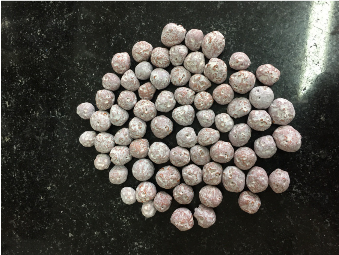
Figure 5.3(a): TiO 2 freshly coated clay beads.
