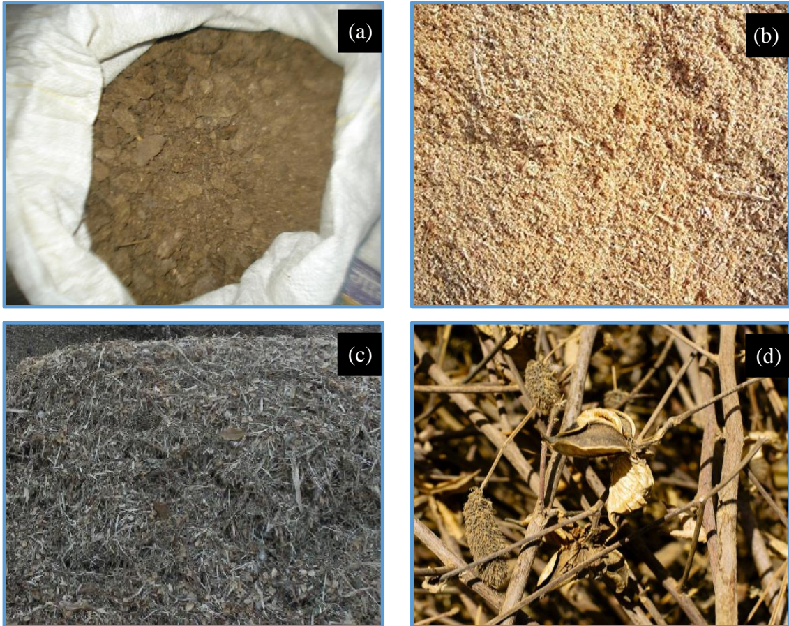
Figure 3.8 Biomass used for gasifier (a, b) sawdust, and (c, d) cotton stalk
