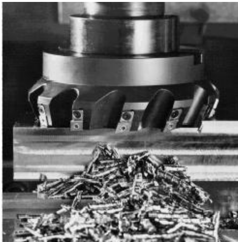
Fig1.6: Face milling operation showing (a) action of an insert in face milling; (b) climb milling; (c) conventional milling d) dimensions in face milling. The width of cut, w , is not necessarily the same as the cutter radius Fig:A face milling cutter with indexable inserts.
