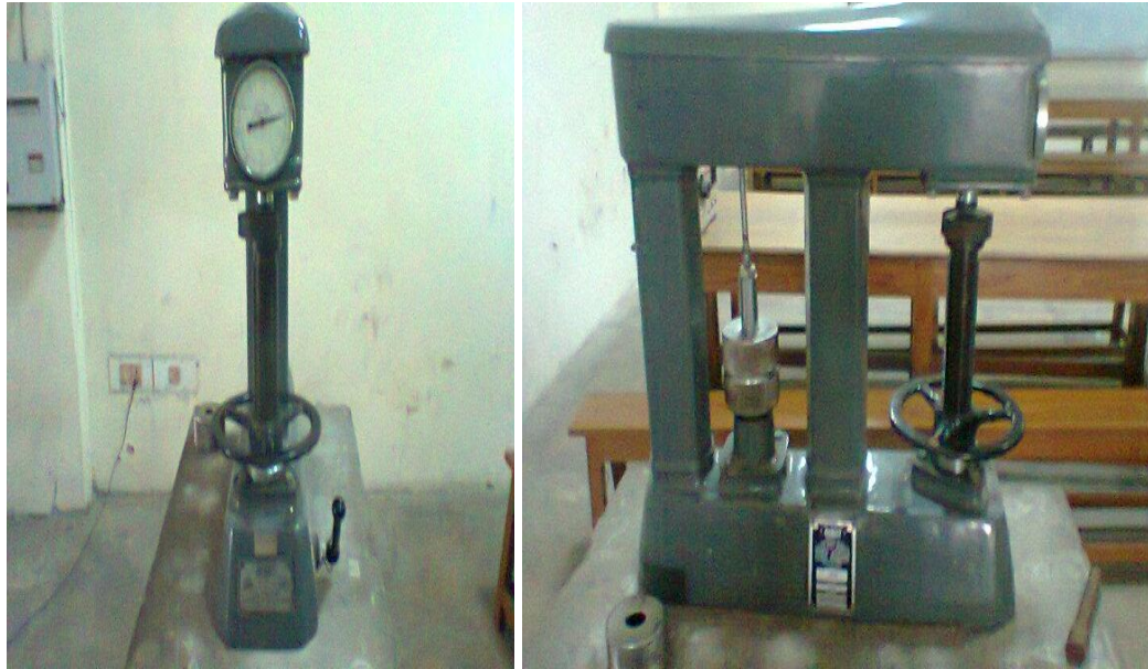
Figure 4.3: Brinell Hardness Testing Machine
