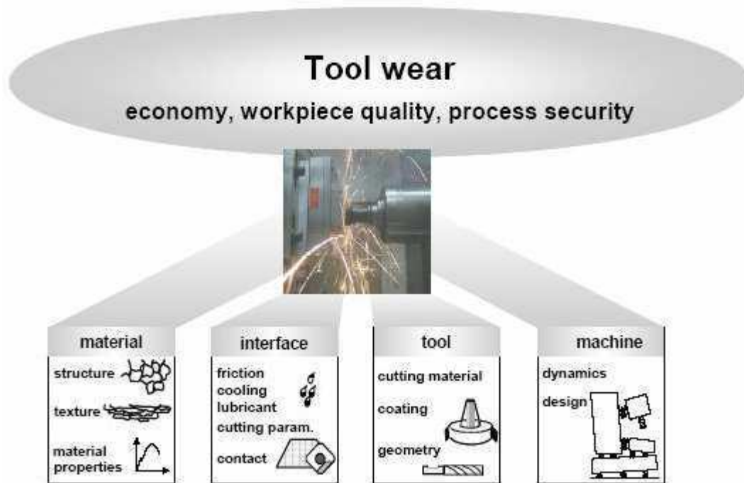
Fig. 1.8 Influencing elements of tool wear
