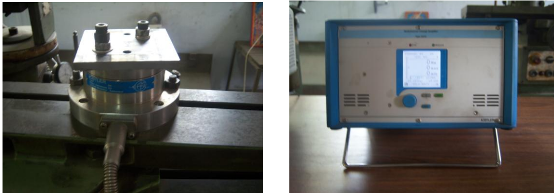
Figure 4.2:- Work piece mounted on dynamometer
