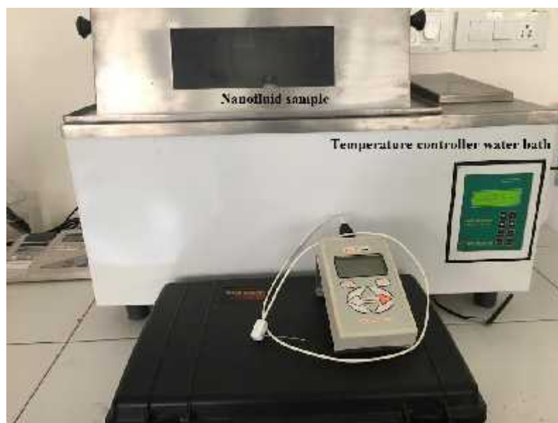
Figure 3.14: Thermal Property analyzer with temperature controller water bath
