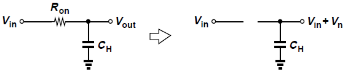
Figure 3.20 Thermal noise in a sampling circuit [1].
