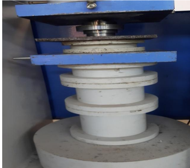
Figure 3.4 Pressing of BaM powder
