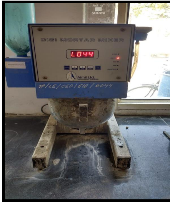
Figure 3.3. Preparation of Cementitious Grout (DG Mixer)
