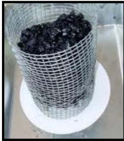
Figure 3.4. Drain Down Test of Specimen
