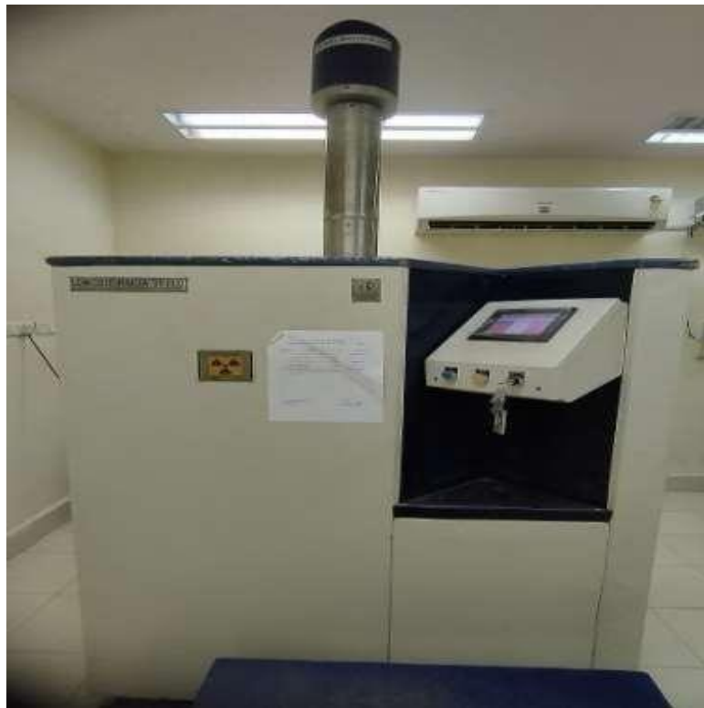
Figure 9: LDI 2000 Co (60)-gamma radiator
