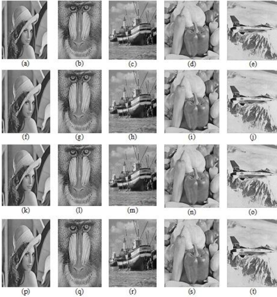
Figure 4.6: (a)-(e) Original cover images; (f)-(j) Marked images after hiding 1,00,000 bits; (k) – (o): Marked image after hiding 5,00,000 bits (p)-(t): Marked image after hiding 10,00,000 bits.
