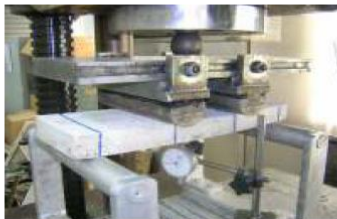
Plate 2.3: Four-Point Load Flexural Strength Test under Progress
