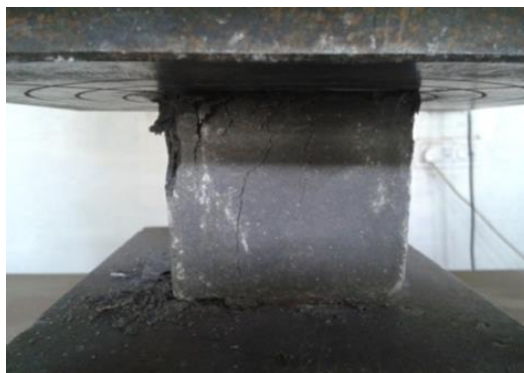
Plate 3.5: Compressive Strength Test on Mortar Specimens in Progress
