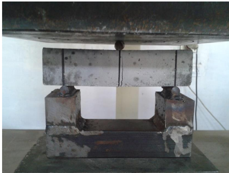
Plate 3.6: Flexure Strength Test of Mortar in Progress
