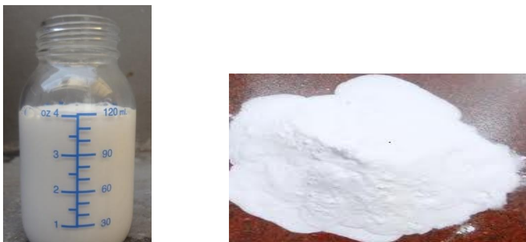
Plate 1.4: SBR Polymer in Liquid Form and VAE Polymer in Powdered Form
