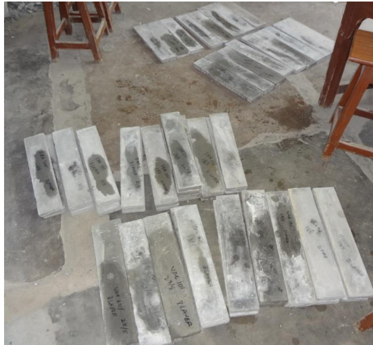
Plate 3.9: Polymer Modified Ferrocement Specimens after Demoulding (before testing)
