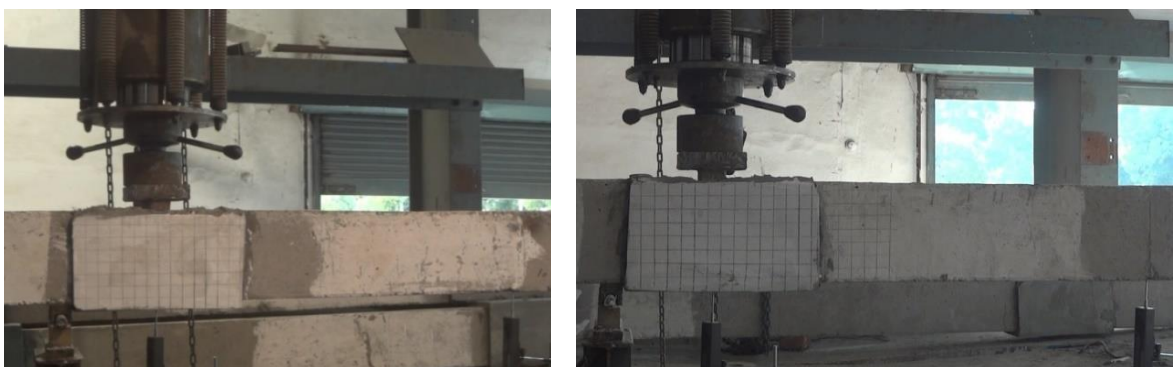
Plate 4.14: Testing of Strengthened RCC Beams in Progress ( a/d = 1.0 )
