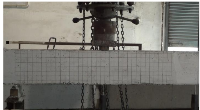
Plate 4.11: Pre-Damaging of RCC Beams at a/d = 3.0
