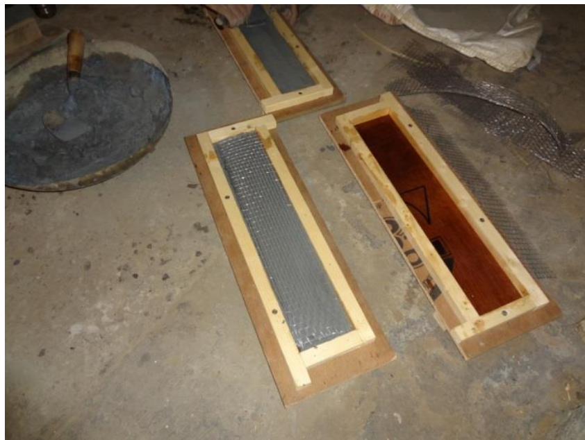
Plate 3.8: Polymer-Modified Ferrocement Specimens under Casting
