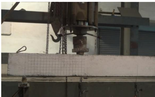
Plate 4.7: Testing of RCC Beams in Progress ( a/d = 3.0 )
