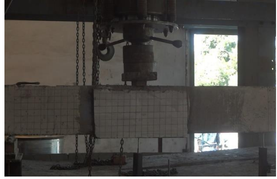
Plate 4.15: Testing of Strengthened RCC Beams in Progress ( a/d = 3.0 )
