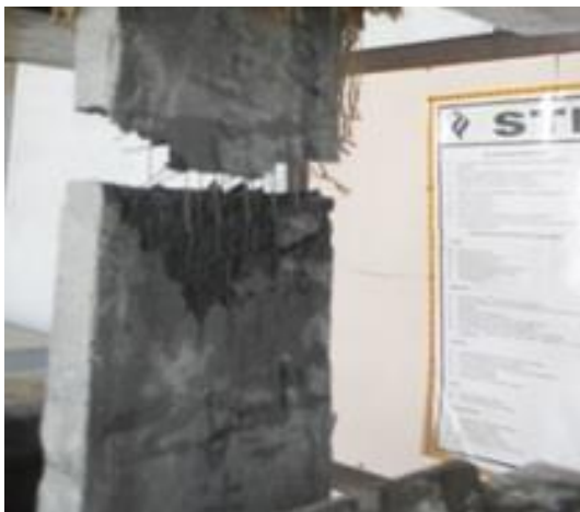
Plate 3.13: Tensile Failure of Ferrocement Elements
