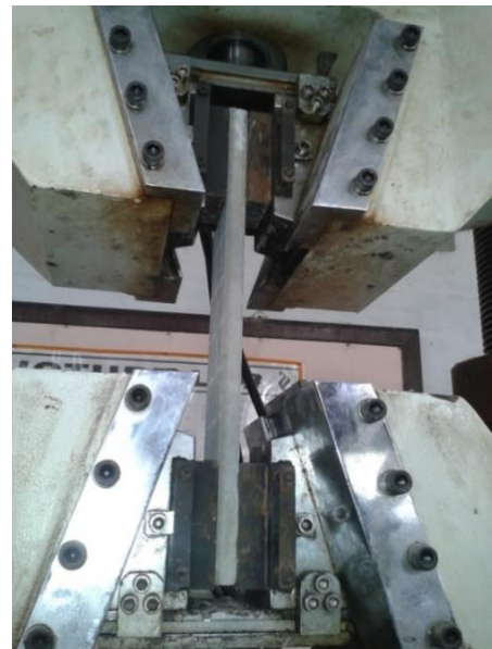
Plate 3.12: Tensile Strength Test of Ferrocement in Progress
