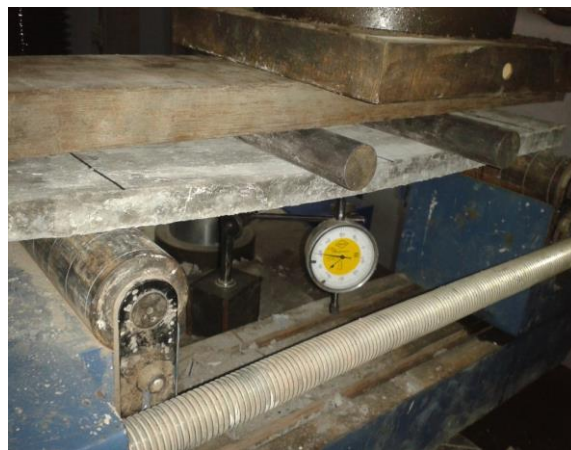
Plate 3.10: Flexural Strength Test of Ferrocement in Progress
