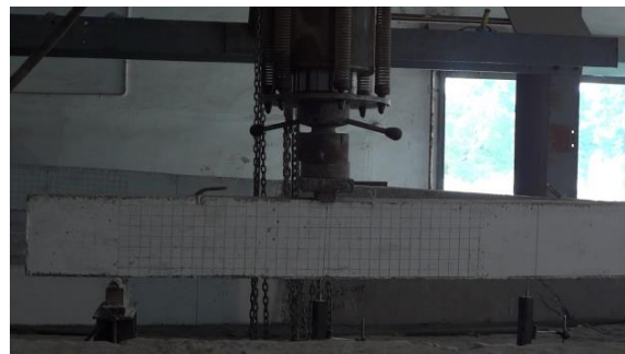
Plate 4.7: Testing of RCC Beams in Progress ( a/d = 3.0 )
