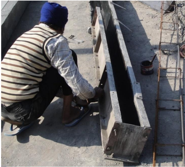
Plate 4.2: Preparation of RCC Beam Specimen (a) Preparation of Steel Formwork; (b) Placement of Reinforcement in the Mould
