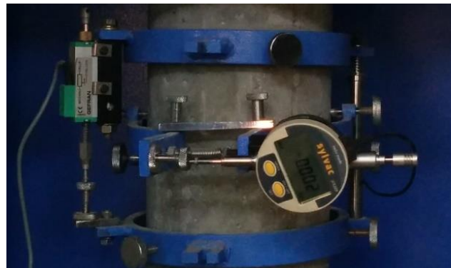
Plate 3.7: Mortar Cylinder during Testing for Modulus of Elasticity
