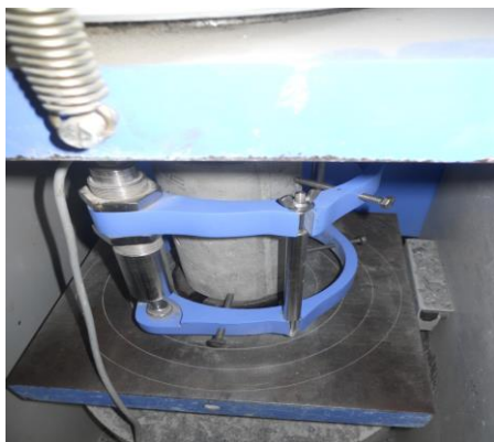
Plate 3.7: Mortar Cylinder during Testing for Modulus of Elasticity
