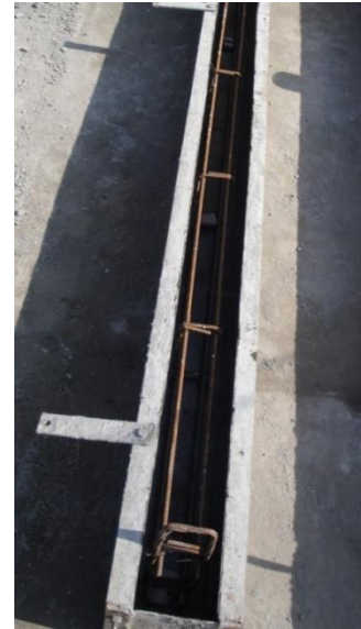
Plate 4.2: Preparation of RCC Beam Specimen (a) Preparation of Steel Formwork; (b) Placement of Reinforcement in the Mould
