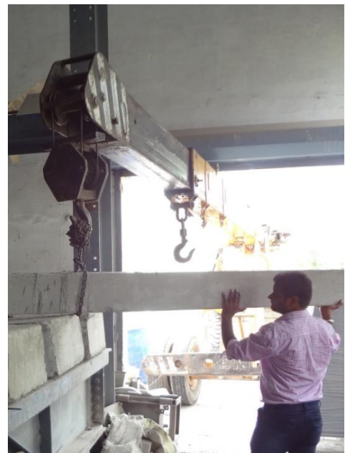
Plate 4.5: Shifting and Placing of Beams on the Loading Frame
