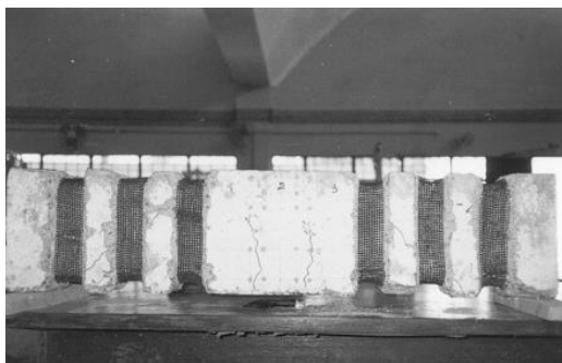
Plate 2.1: Detail of Beam Strengthened by Ferrocement Strips in Shear Span
