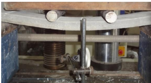
Plate 3.11: Flexural Failure of Ferrocement Elements
