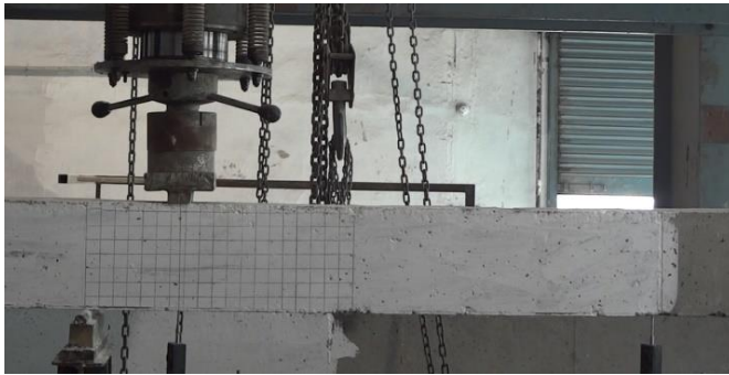
Plate 4.10: Pre-Damaging of RCC Beams at a/d = 1.0
