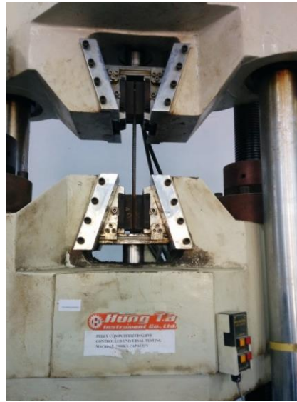
Plate 4.1: Testing of Reinforcement Bars
