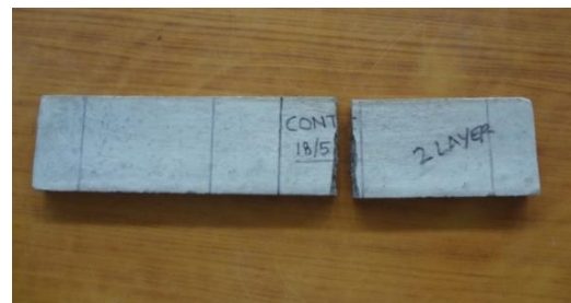
Plate 3.11: Flexural Failure of Ferrocement Elements
