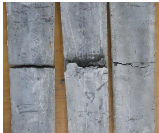
Plate 3.13: Tensile Failure of Ferrocement Elements
