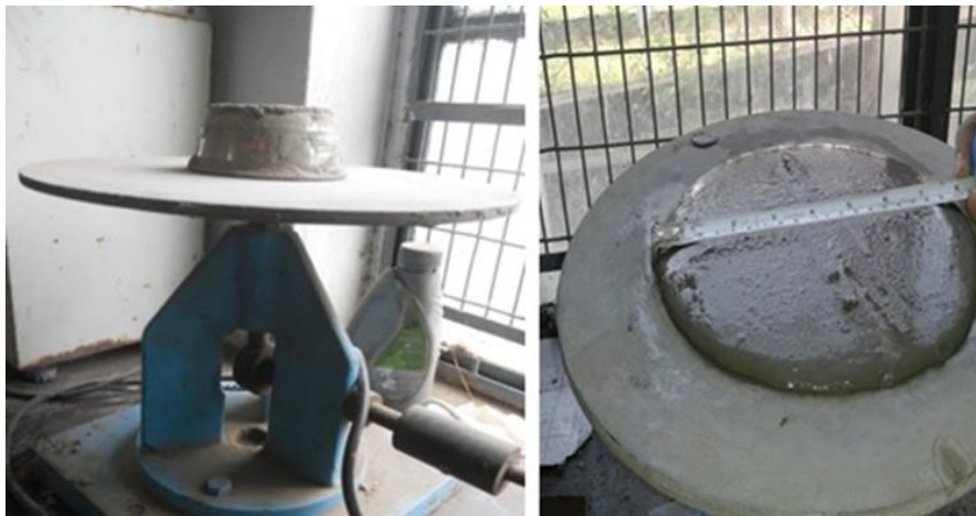
Plate 3.3: Flow Table and Measurements of Flow Value of Mortar
