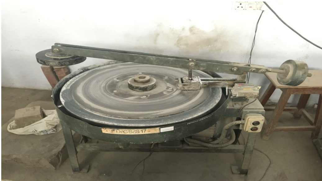
Figure 3.15: Abrasion testing machine used in the study
