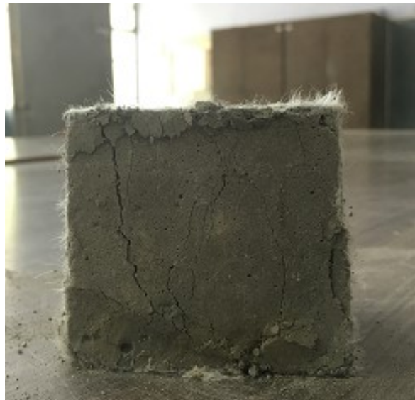
Figure 3.8: SHCC cube tested for compression
