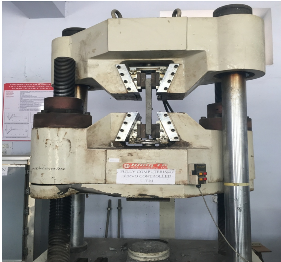
Fig 3.14: UTM used for the tensile test
