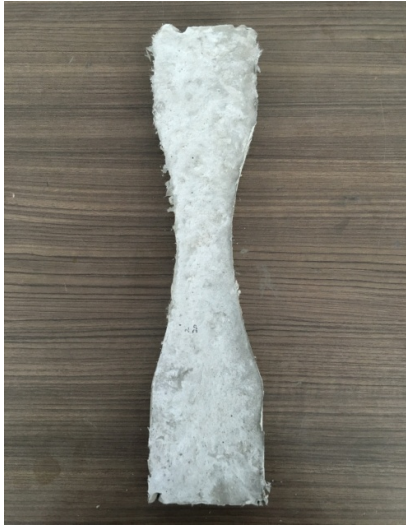
Figure 3.12: Casted sample of SHCC
