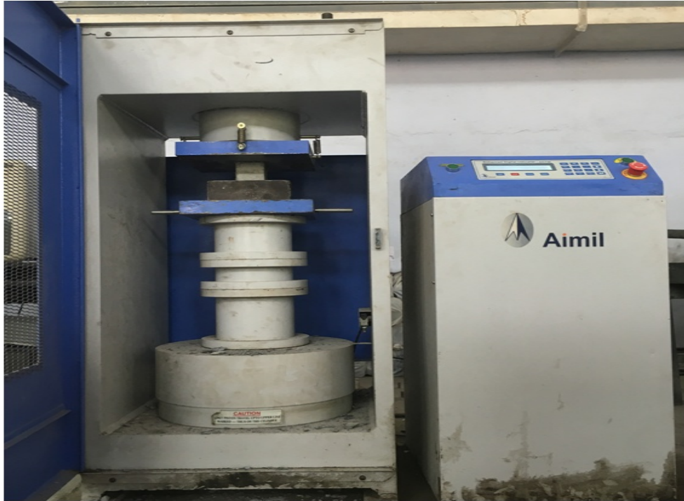
Figure 3.7 Compression testing of sample of SHCC.
