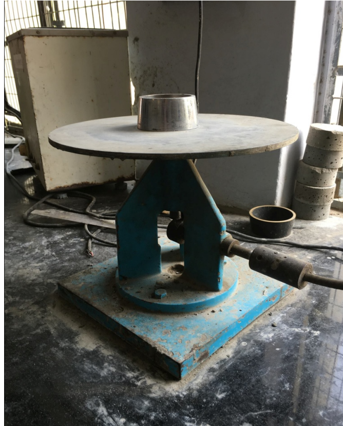
Figure 3.10: Flow table machine used in the study
