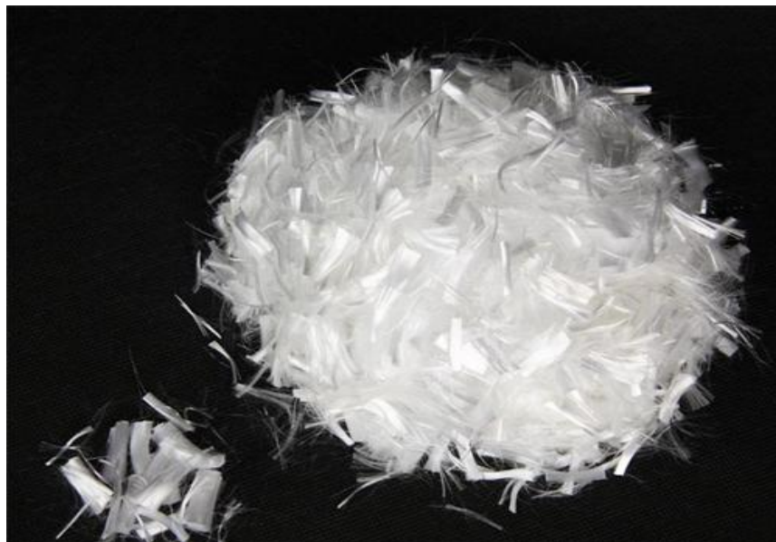
Figure 3.6: PVA fibers used in the study
