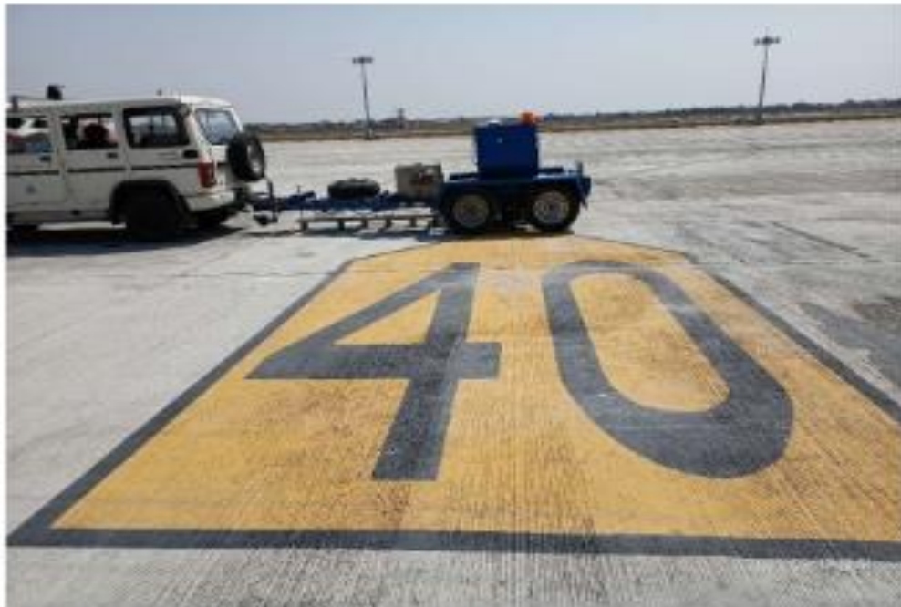
Fig 5. 5 Heavy deflector testing in progress on Stand 40 Rigid.
