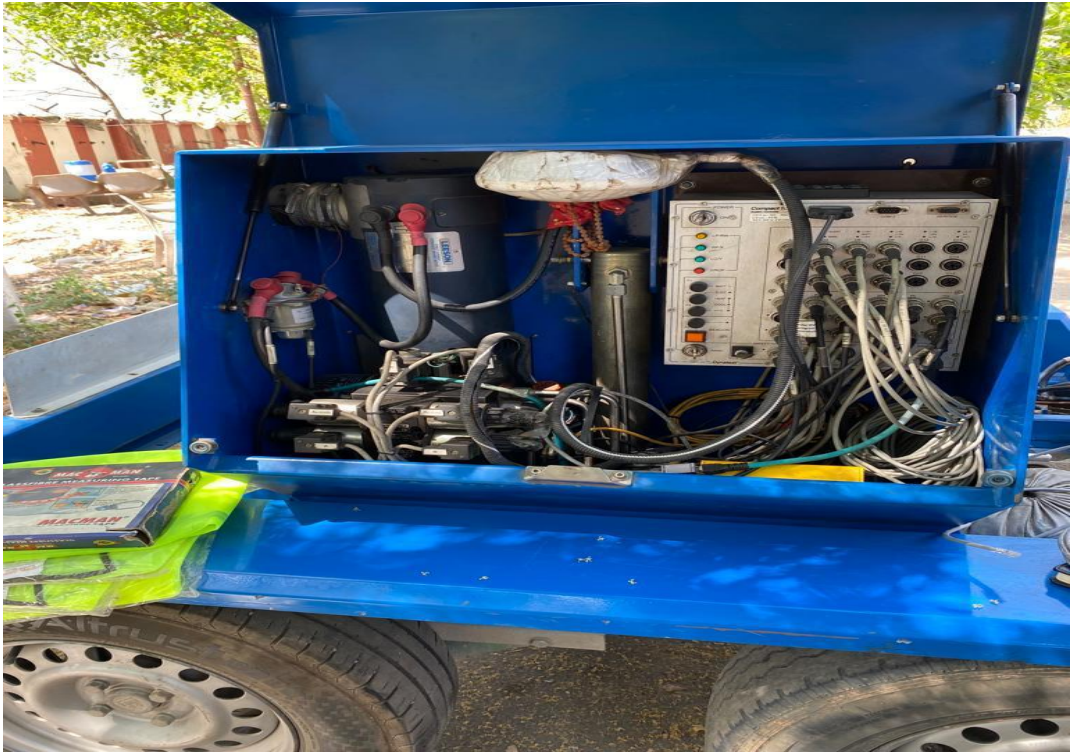
Fig 3. 10 Control Box of the FWD device
