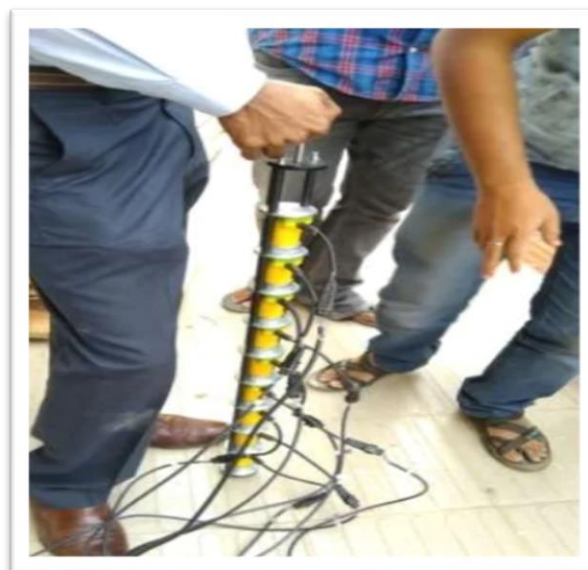
Fig 3. 8 Stack test for Calibration of the Geophones.
