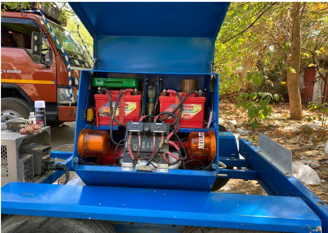
Fig 3. 11 Battery Box and GPS setup of the FWD device.
