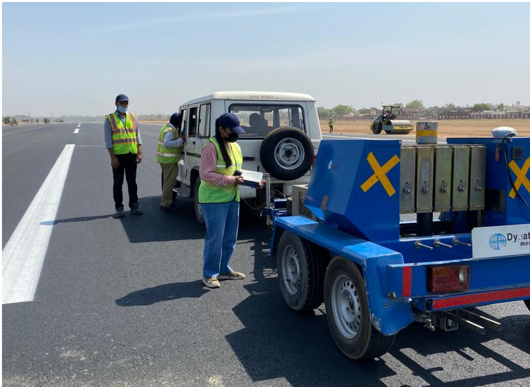
Fig 5. 7 Heavy Weight Deflectometer testing in progress on Runway (Ab-Cd)
