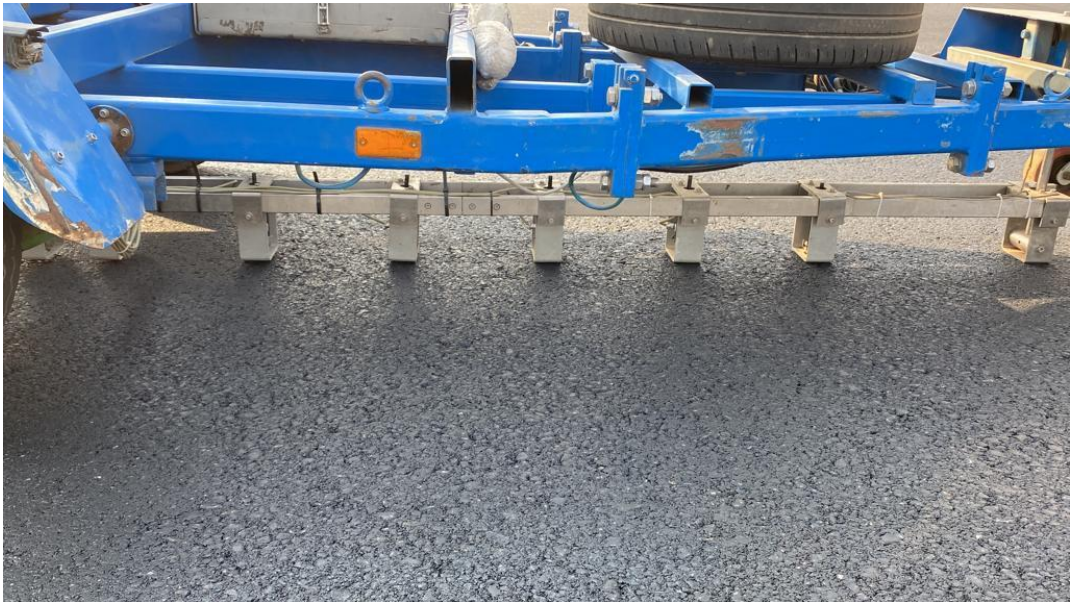
Fig 3. 13 Sensor bar in contact with the pavement surface
