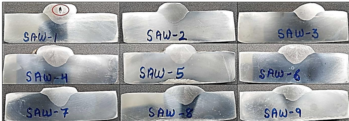
Figure 6.5: Macrostructure of SAW coupons (1 To 9)
