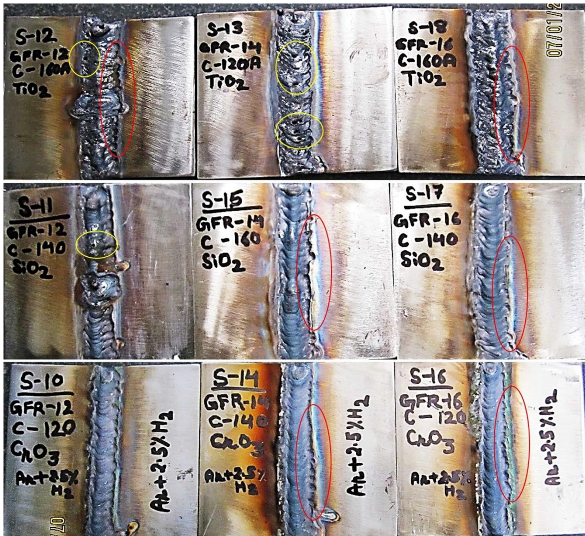
Figure 5.5: Weld bead appearance of Ar shielded weld coupon (S-10 to S-18)
