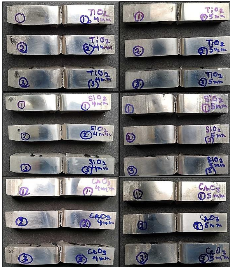
Figure 8.19: Etched and Tested samples of toughness test (Charpy) show the penetration profile
