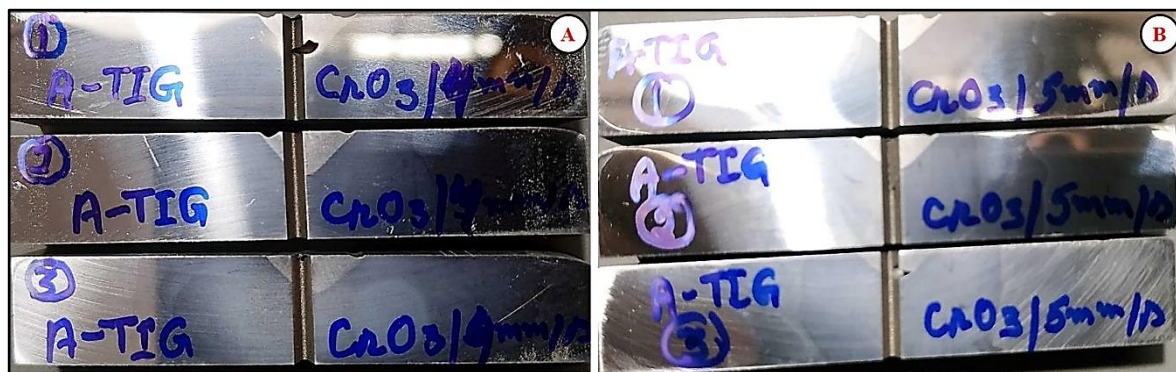
Figure 7.5: Showing extracted, the polished and etched specimen of toughness test (Charpy) (A) AA – TIG_ \text{CrO}_3 _4 mm/s and (B) AA – TIG_ \text{CrO}_3 _5 mm/s
