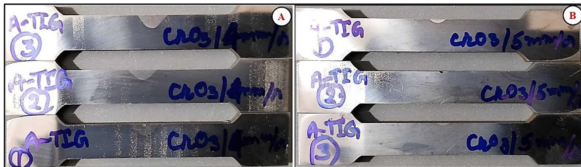
Figure 7.8: Extracted specimen from AA – TIG welding (A) AA – TIG_CrO 3 _4 mm/s (B) AA – TIG_CrO 3 _5 mm/s
