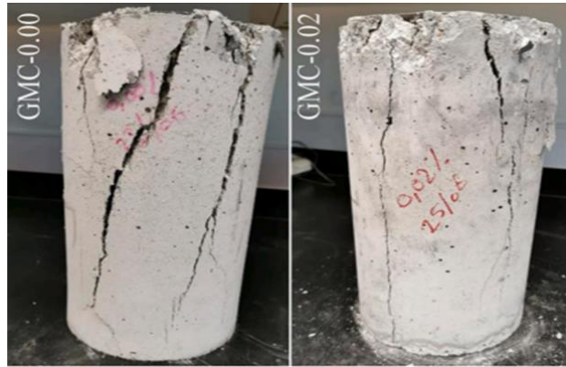
Figure 2.1 Crack width in Specimens with respect to GNP % (Ismail et al. 2022)
