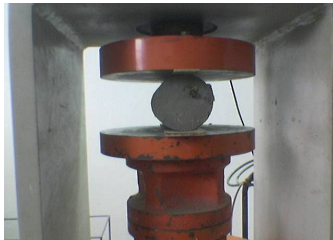
Fig. 4.2 Split Tensile Strength Test
