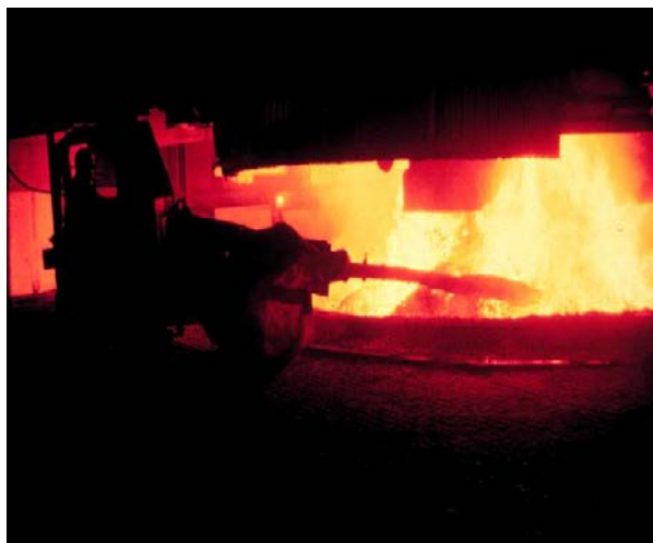
Fig 1.5 Charging deck of the furnace
