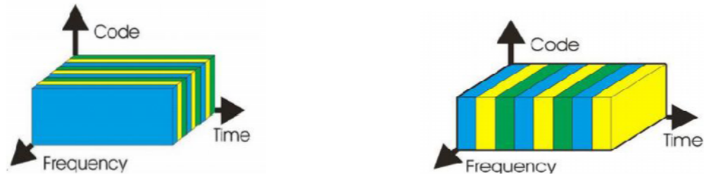
Figure 1.1: a) Channel usages by WDMA or FDMA b) Channel usages by TDMA [6]
