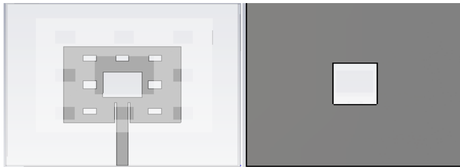
Fig 4.2 Figure showing geometry of Patch and DGS based ground plane
