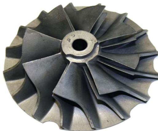
Fig. 11 Two plane balancing of an impeller on nose and back-face (Books, 2015)
