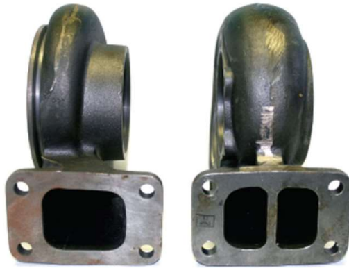
Fig. 26 Tangential entry single and twin entry turbine housing (Books, 2015)
