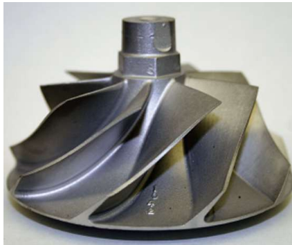
Fig. 13 Full blades of an impeller (Books, 2015)
