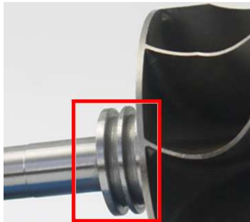
Fig. 32 Twin seal grooves for two seals (Worldturbocharger.com, 2018)
