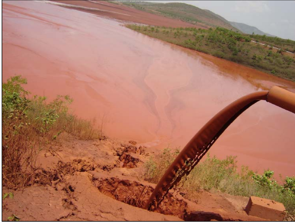
Fig 1.3: Disposal of red mud in the form of wet slurry to nearby artificial impoundment at NALCO, Damanjodi, Orissa, India
