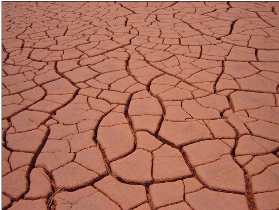
Fig 1.4: Red mud ponds are left open for sun drying, leaving cracks after being dried at NALCO, Damanjodi, Orissa, India
