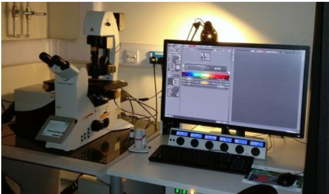
Figure 24: Leica TCS SP8 confocal microscope has been designed with optimal photon efficiency and high speed. This system has 3 detectors (1 sensitive Hybrid GaAsP and 2 PMT) and a motorized XYZ-stage
