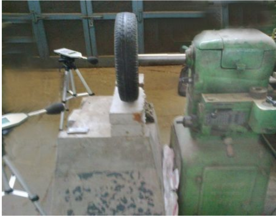
Figure32 Experimental set-up, without any preventive measures, for background noise estimation
