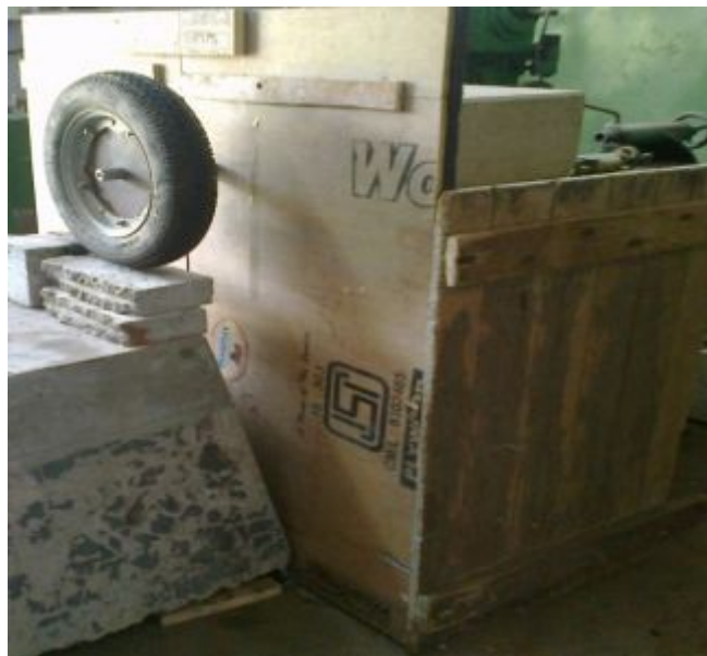
Figure 34 wooden walls for shielding of remaining background noise
