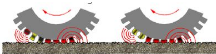
Fig.18 Radial and tangential vibrations of the tire tread [26]
