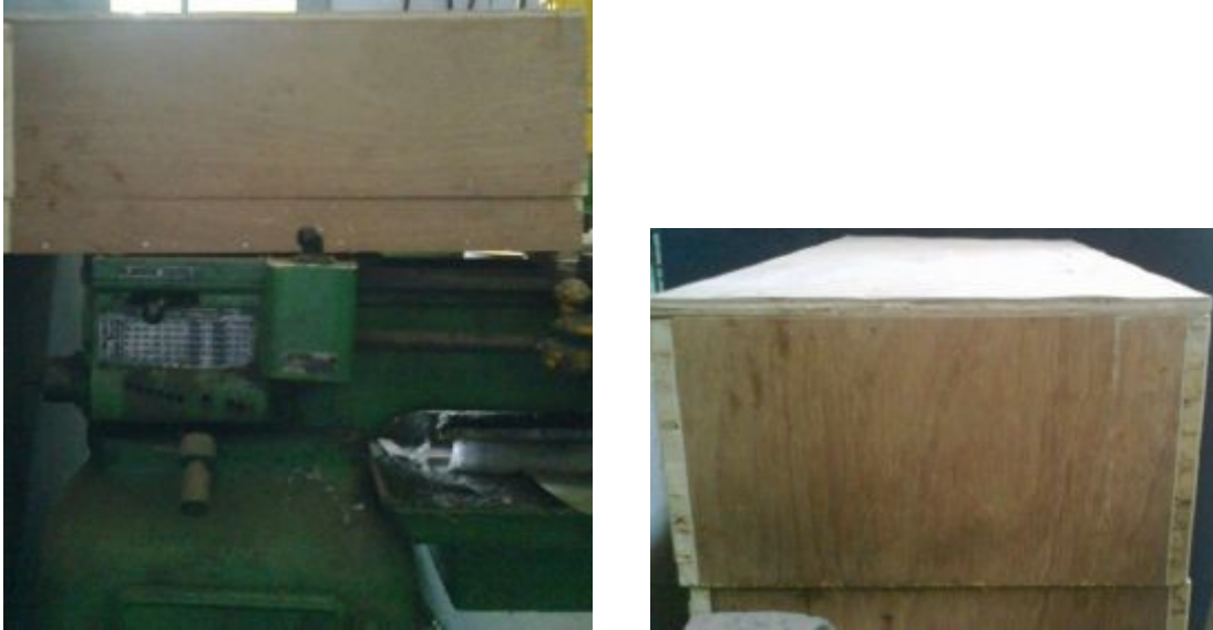
Figure33 wooden box for shielding of moving parts of experimental rig
