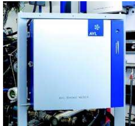
Figure 7(a): Smoke meter working principle [28] Figure 7(b): Smoke meter unit [28]
