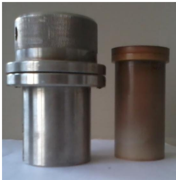
Figure 2.2 Teflon lined stainless steel cylinder
