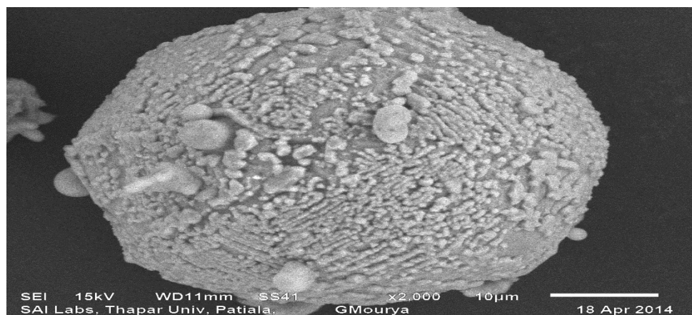
Fig.4.13 SEM image of S-I bottom ash leachate
