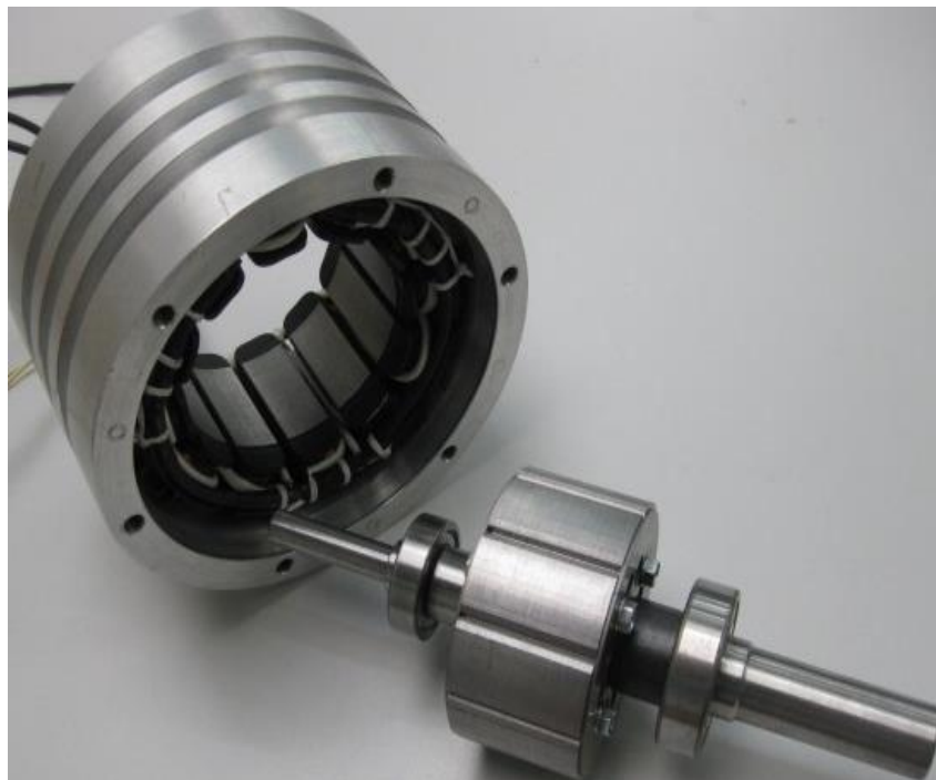
Figure-3.1: Construction of PMSG
