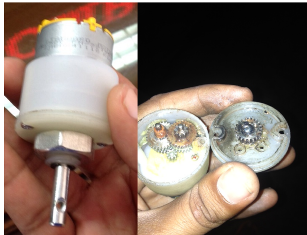
Figure 4.13: DC geared motor inside view
