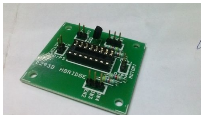
Figure 4.15 L293D motor driver
