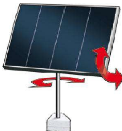
Figure 1.5: Dual axis tracker [5]
