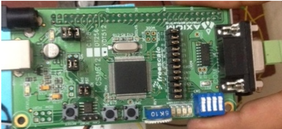
Figure 4.19: MCU9S12XDT512 Freescale micro-controller
