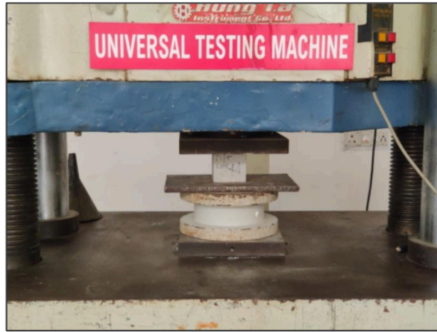
Figure 3.12 Experimental setup employed for determining the compressive strength of mortars.
