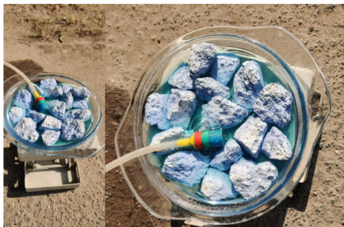
Figure 3.18: Batch experimental setup for evaluating the photocatalytic performance of the \text{Fe}_2\text{TiO}_5 heterostructure for cementitious composite.
