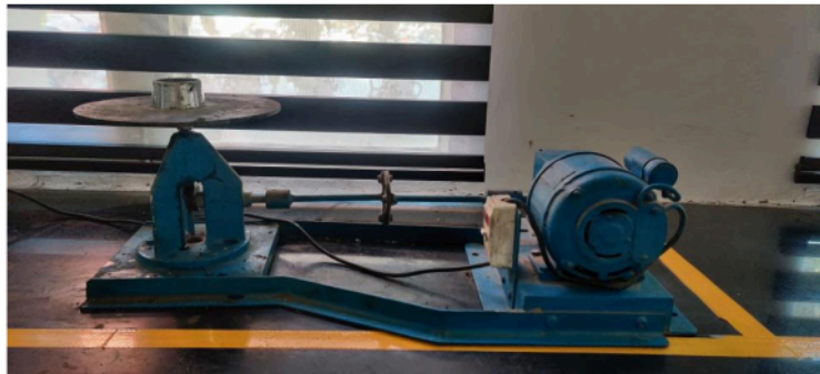
Figure 3.10 Apparatus for determination the workability using slump flow test.
