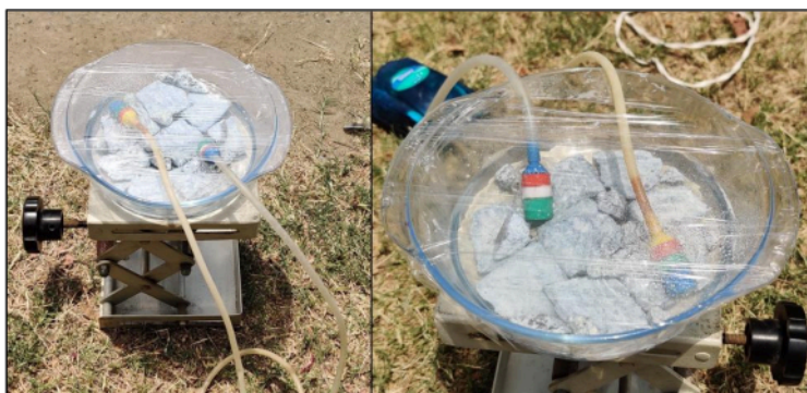
Figure 3.19 Batch experimental setup for evaluating the antibacterial property check of the Fe 2 TiO 5 heterostructure composite.
