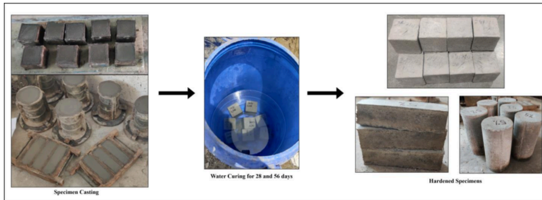
Figure 3.9 Various stages while casting different design mixture (C x S y ) hardened specimens.
