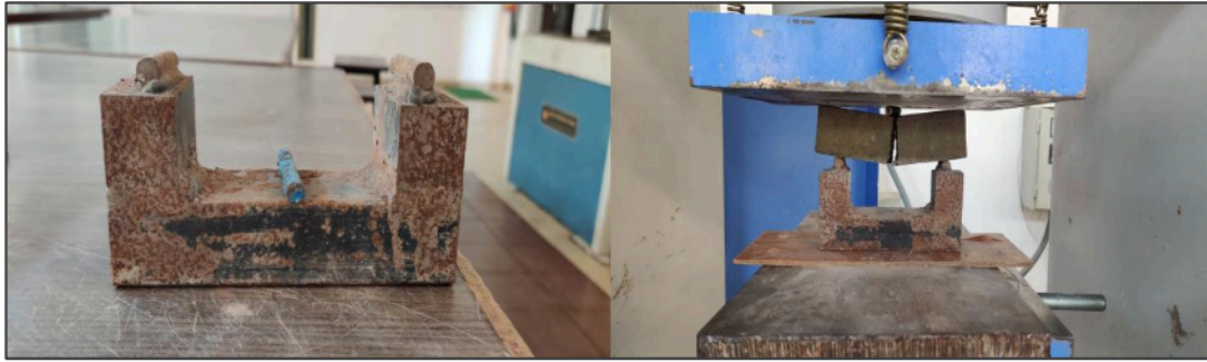
Figure 3.13 : Experimental setup employed for determining the flexural strength of the prism specimens.
