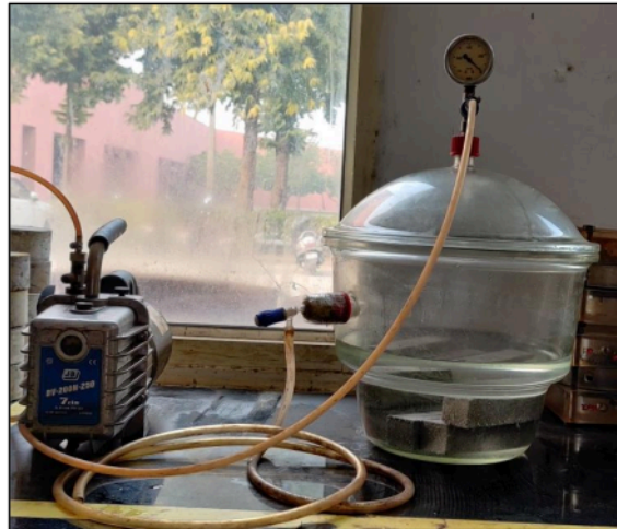
Figure 3.15 Samples placed in a desiccator containing water under atmospheric pressure.
