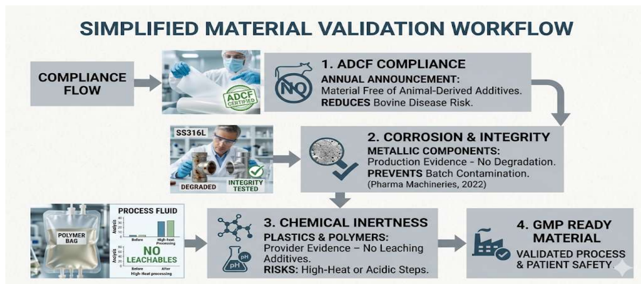
Figure 3 -Material validation workflow (Shukla & Gottschalk, 2013).
