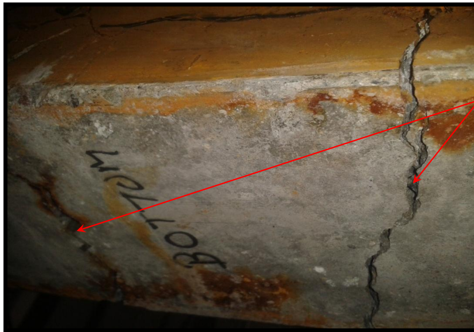
Fig: 5.30 C-28 Beam showing cracks at soffit after failure
