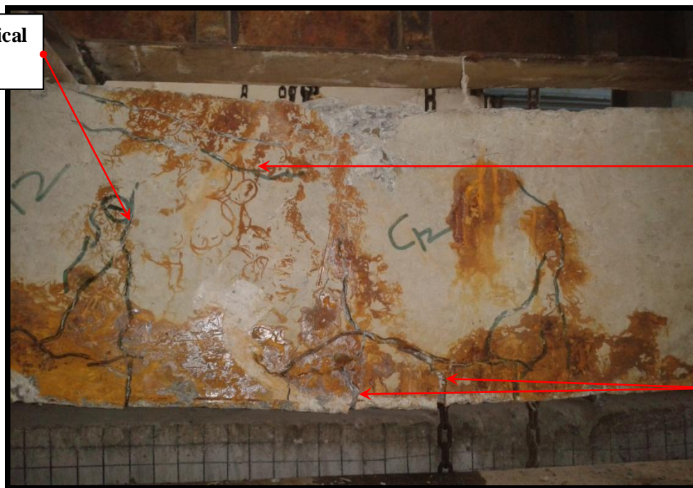
Fig: 5.21 Side face of C-12 Beam showing cracks after failure
