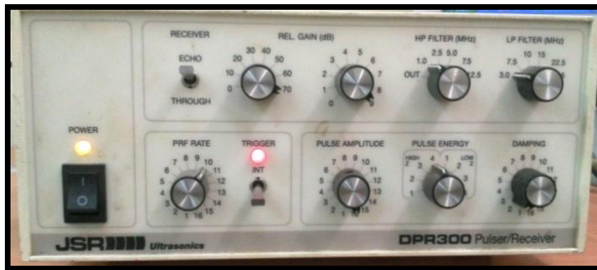
Fig: 4.10 pulser/receiver (DPR 300, JSR Make)
