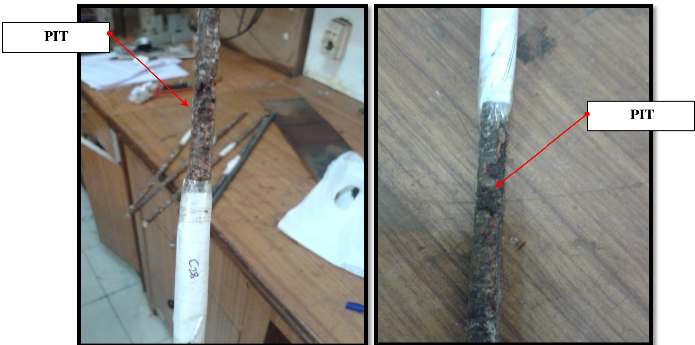
Fig: 5.40 Closure View of Pit formation
