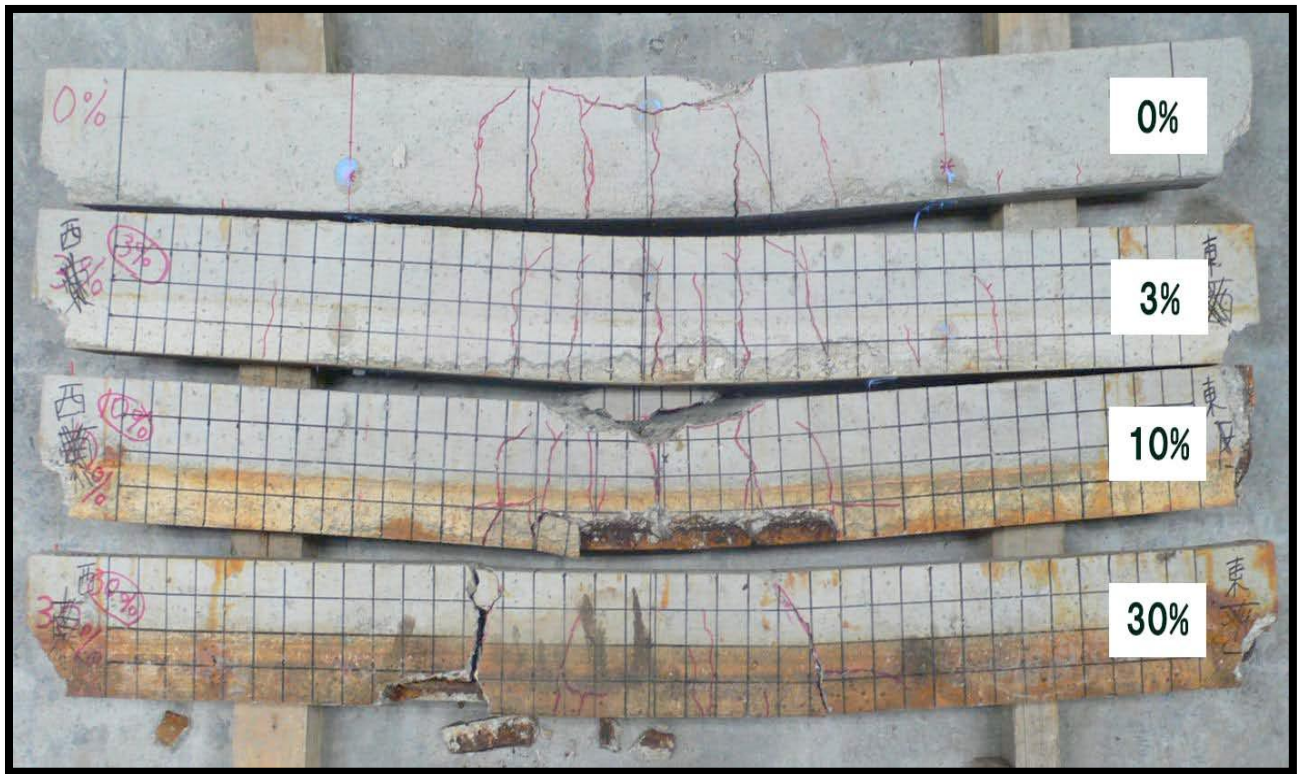
Fig: 3.15 Crack patterns after loading tests Okude et. al., (2009)
