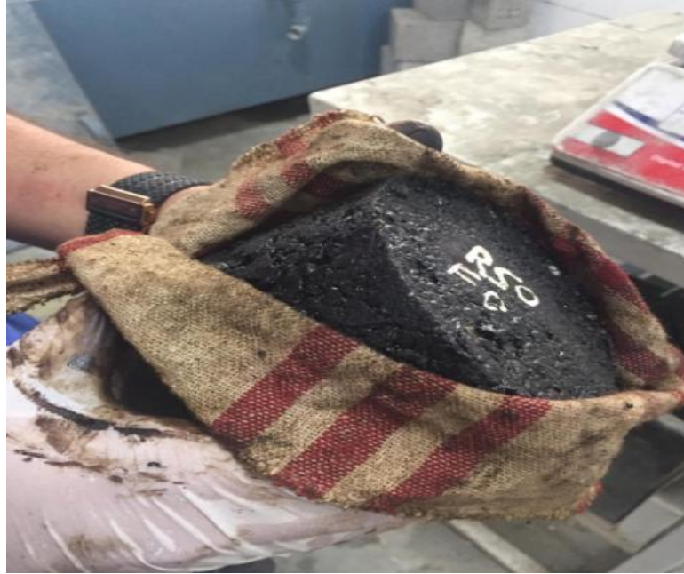
Figure 3.13: Saturated Surface Dry weight of specimen(SSD).
