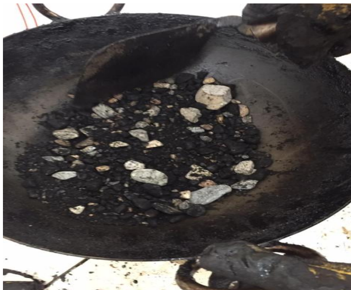
Figure 3.7: Mixing of marshall sample
