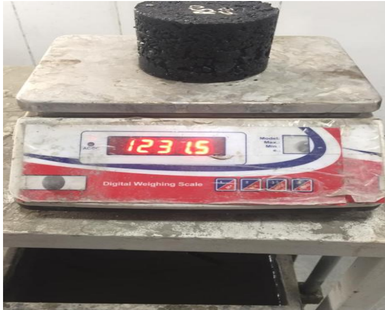
Figure3.11: Dry weight of Marshall Specimen.
