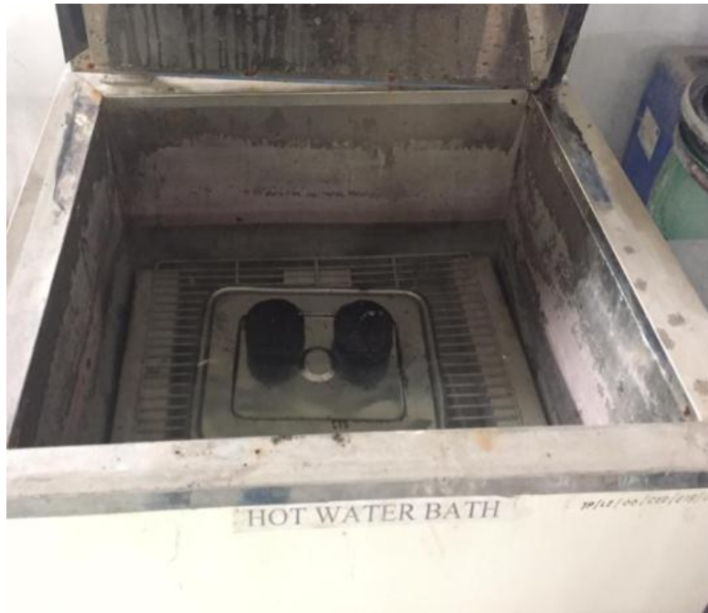
Figure 3.14: Specimens are kept in Hot water bath at 60°c.
