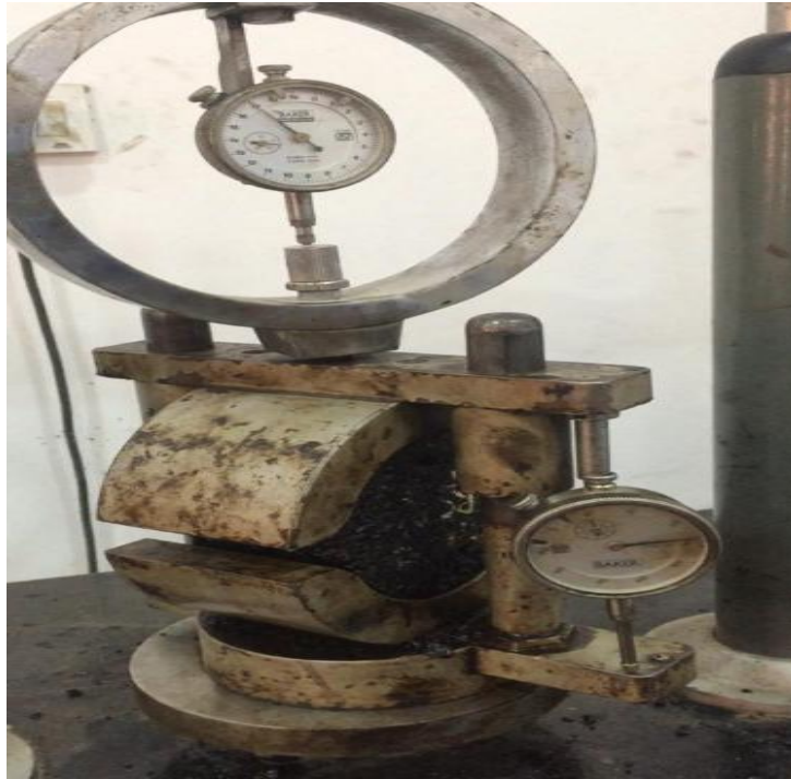
Figure 3.15: Marshall Flow and Stability testing.
