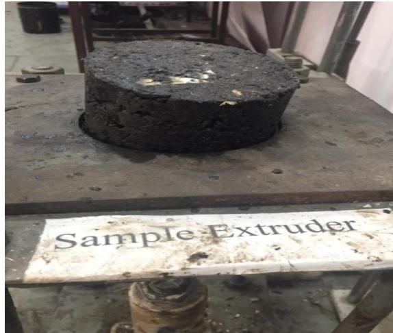
Figure 3.10: Extraction of Marshall Specimen.
