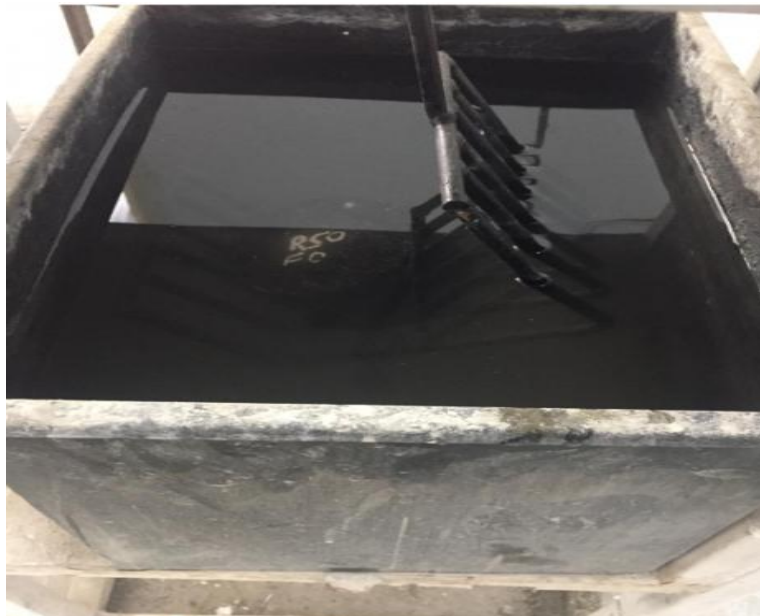
Figure3.12: Submerged weight of specimen.
