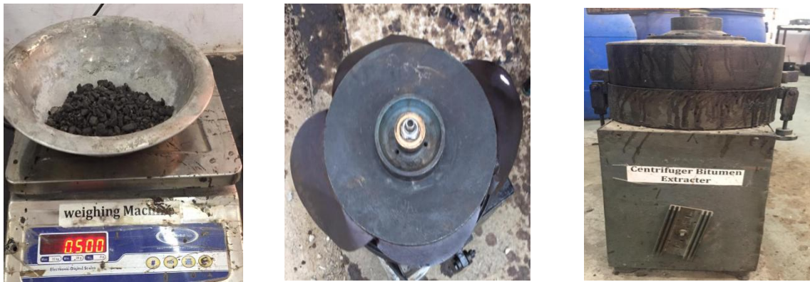
Figure 3.3: Bitumen extraction using centrifugal extractor.
