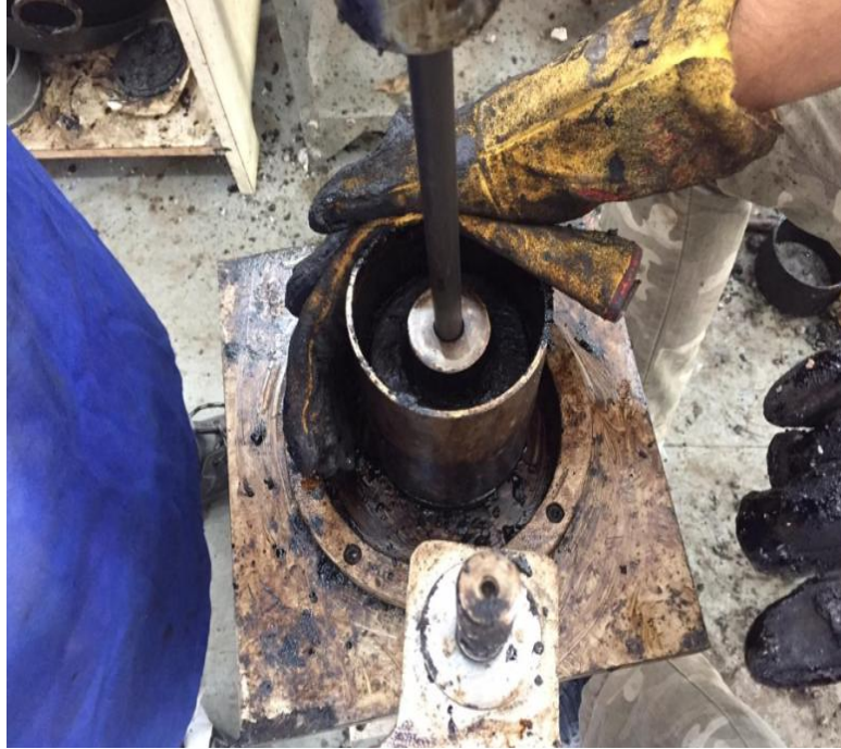
Figure 3.8: Applying 75 blows on marshall mould
