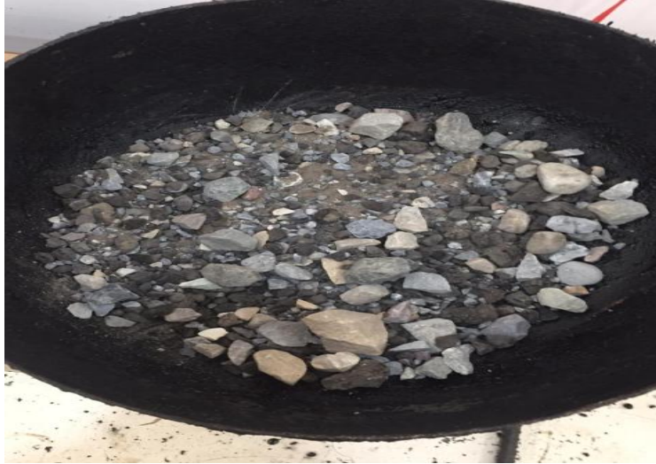
Figure 3.6: Marshall grading of aggregates.
