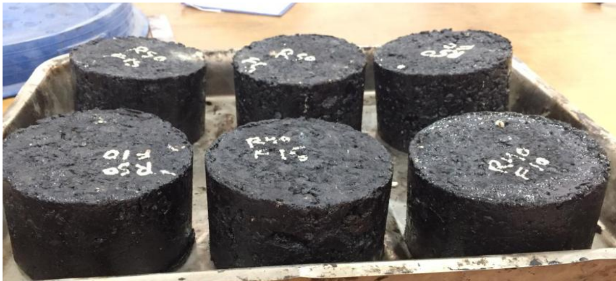
Figure 3.5: Prepared Marshall Specimens with different RAP contents
