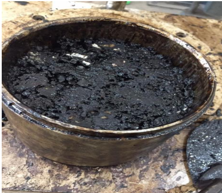
Figure 3.9: Allow specimen to cool down for 24 hour.
