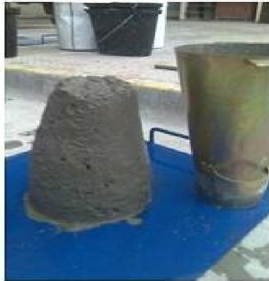
Figure 4.2 Slump for RAC 100 %
