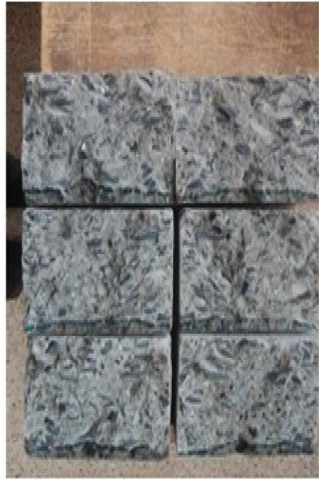
Figure 3.14 Water penetrated Sample
