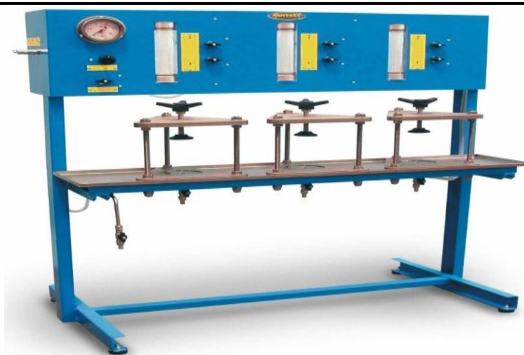
FIGURE 3.12: Water penetration test
