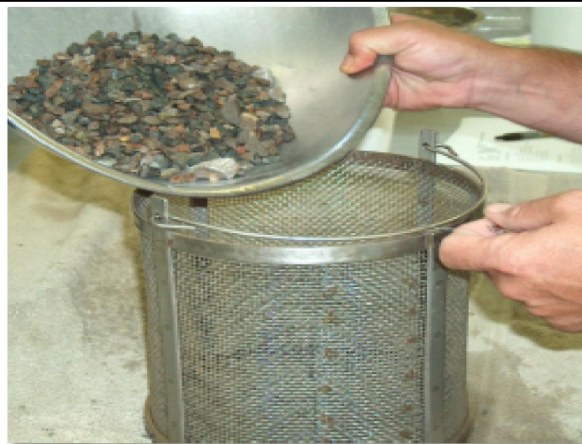
Figure 3.2: bucket method used for measuring specific gravity of aggregate
