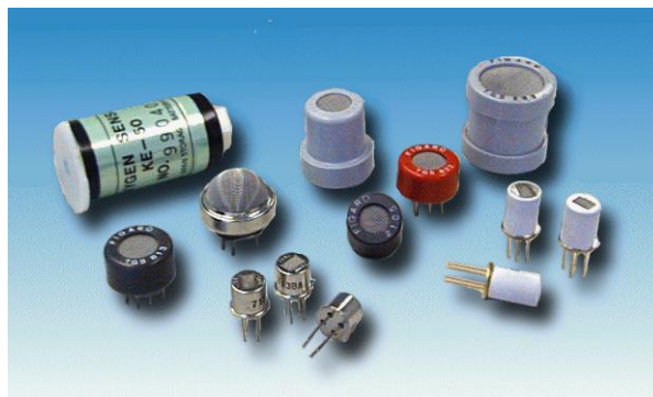
Fig. 1.1: Different commercially available single sensors using semiconductor technology, Figaro Engineering
