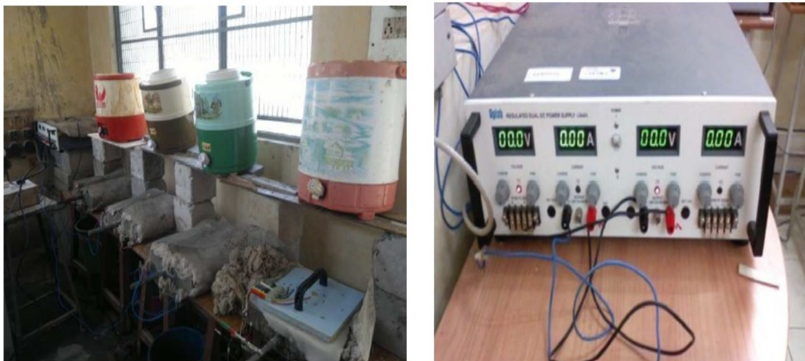
Fig 4.2 Specimens and the Power Supplies used to accelerate corrosion
