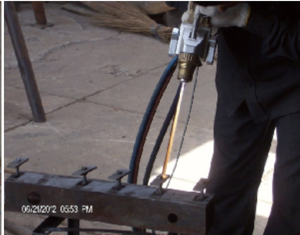
Fig 4.11 HVOF coating process used for the coating of specimen
