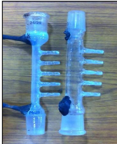
Figure 4.8: Photographic view of pipes; (ID = 10 mm and 20mm).
