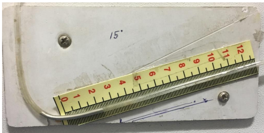
Figure 5.11: Inclined manometer at 15°
