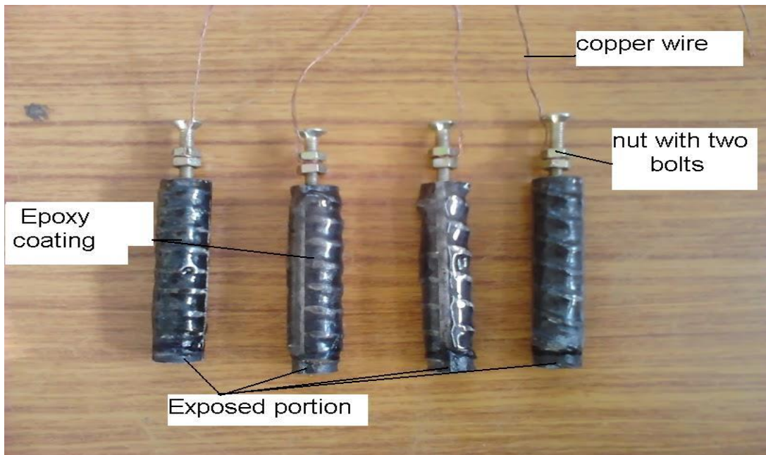
Plate 4.1 Steel specimens with epoxy coating
