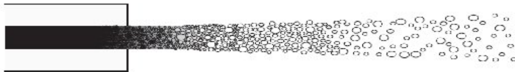
Fig.2.13: Airless atomization with fluid under pressure.
