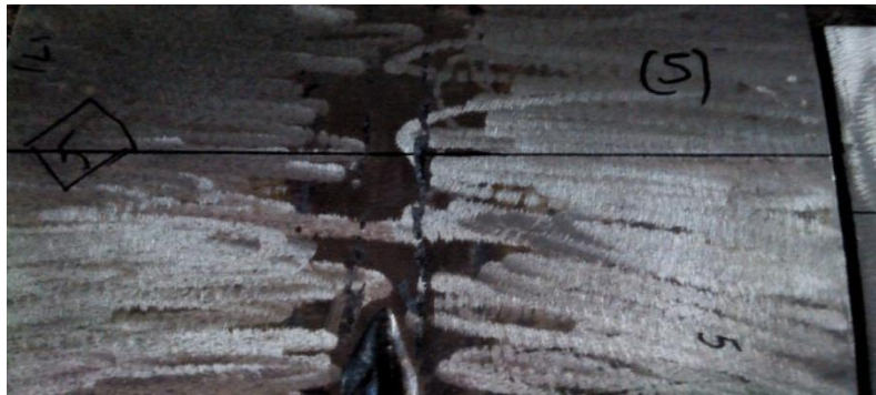
Fig. 4.10: Plates after grinding from weld area
