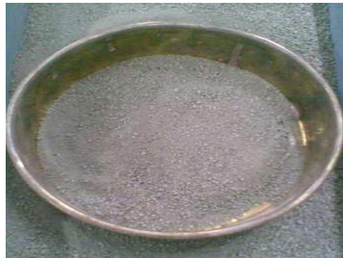
Fig. 4.4: Test sieve (8 BS, 10 ASTM, 2 mm IS, 2057 micron)
